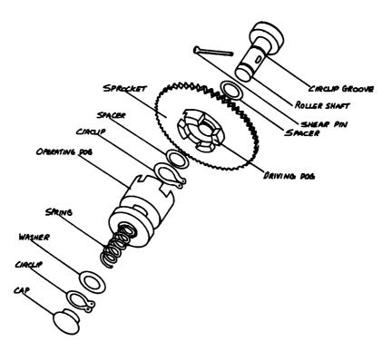
Fig. 15. An exploded drawing.
