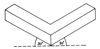
Fig. 14. An isometric drawing.
